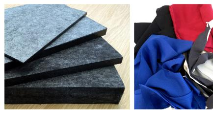
High-Press Fibre Panel comes in various sizes, density and thickness to cater for different purposes from wall panel, roof insulation, flooring, etc. (left), polyester offcuts are the only material that makes this versatile panel (right)
