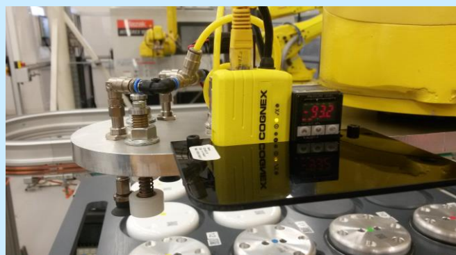
QR Reader on the robot end effector
