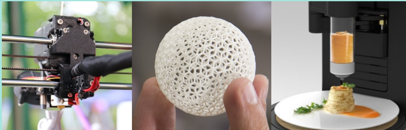
Figure 13. As exemplified by Mortara and Flammini (2018), two core features of 3D printing (left image) include (1) the precise deposition of a range of materials (2) in designated locations. These features afford designers to make intricate structures using composite materials (central image). Additionally, looking towards the future, this technology holds the potential to afford the on-the-spot creation of complex dishes (right image). Images sources (left to right): Lucie Siegelsteinová on Unsplash, metalurgiamontemar0 on Pixabay, Creative Machines Lab, Columbia University.
