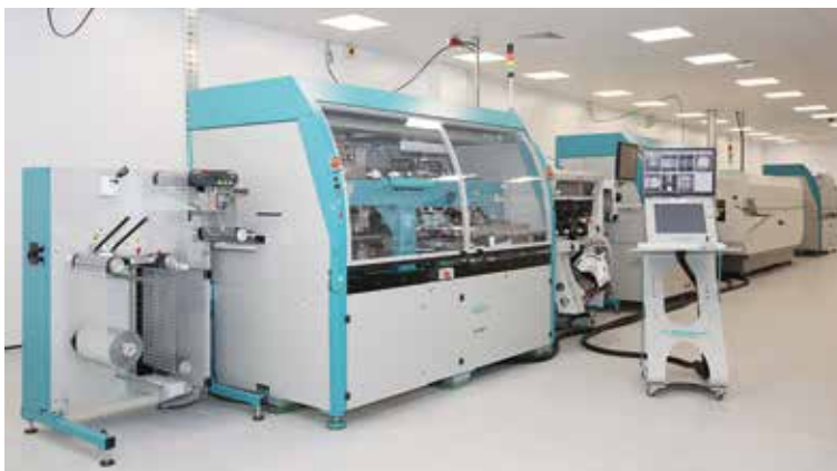
Left: The R2R integration tool integrates electronic chips on to a flexible substrate. Right: The ReMediES NFC smart label.
