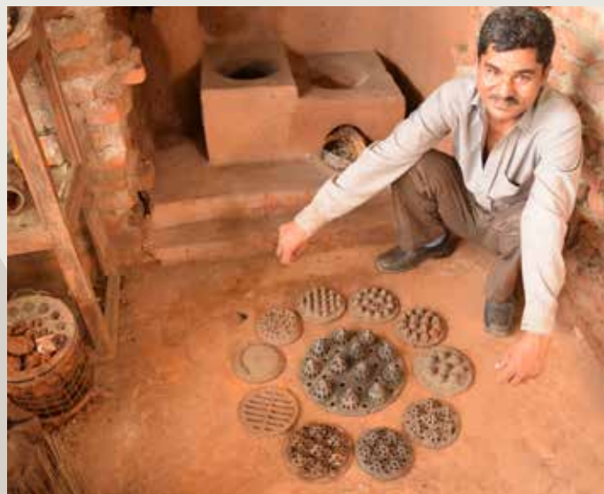
Cookstoves: 10 years' worth of iterative development of burner design
