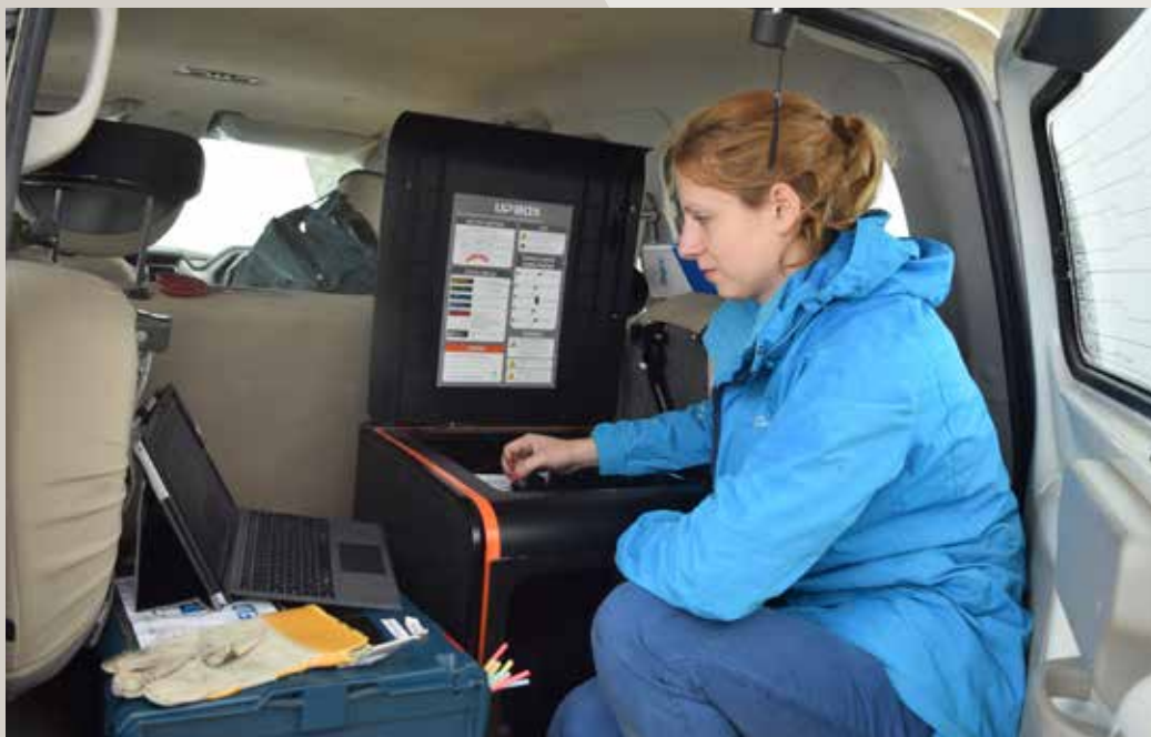
Abi Bush printing a fetoscope (used to listen to an unborn baby's heart) for a health post in an Internally Displaced Persons camp in Nepal.
