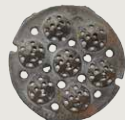
3D printed pattern for burner (top) and final cast iron burner
