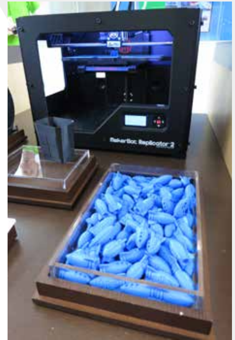
Skype 'rockets' produced by a 3D printer in a US Microsoft retail outlet. Each one takes 20 minutes to produce.
