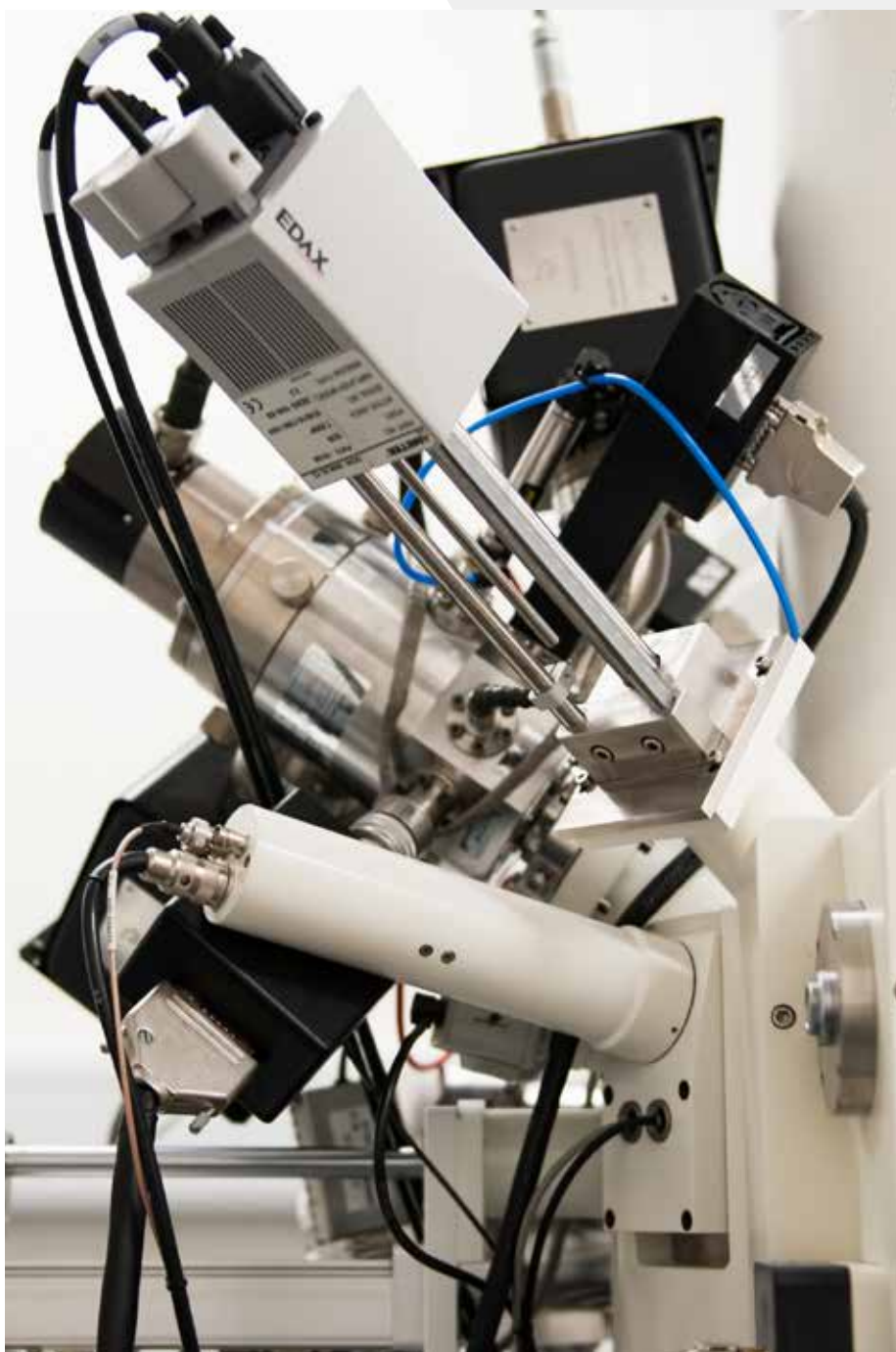
Focused Ion Beam (FIB) microscope which can image and machine materials at a scale of 10nm.
