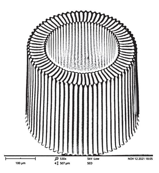
Fun with electrochemically active micro-structures! Thousands of carbon nanotubes are grown closely together to form a cone that can be opened and closed using an electrical charge.
