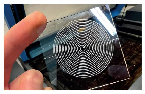
Structures patterned into touchscreen glass increases their sensitivity as sensors. The spiral pattern is excellent for measuring droplets.
