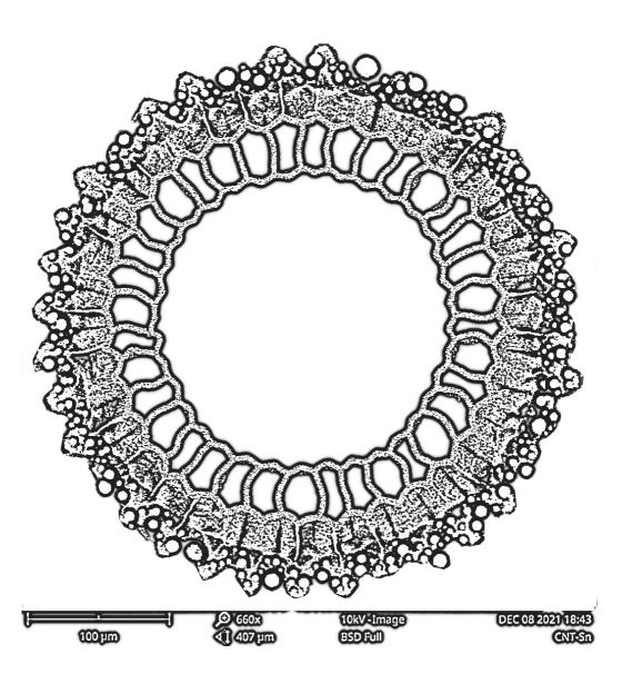
Changing the pattern the nanotubes are grown in changes the cone structure and how it behaves inside new batteries.
