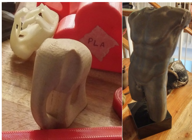
Figure 27: 3D printed shape of an elephant with PLA-wood (left) and a torso printed with PLA-bronze (right), both shown in the iMakr store in London.
