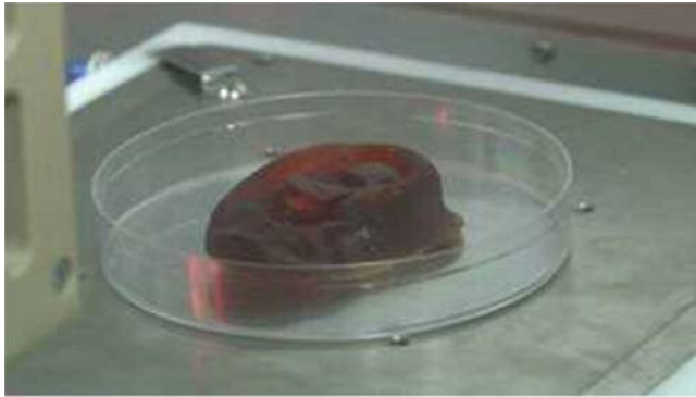
Image: High resolution ear structure bioprinted (this was a biologically inert structure).
