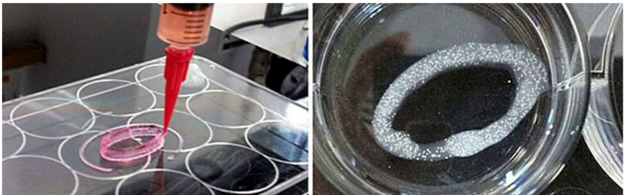
Image: A tracheal pre-tissue produced using 3D Bioprinting and the resulting Chondrocyte-based tissue after two days of maturation.
