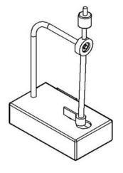
The pendulum blister pack and transport jig will be made using Rapid Proto Type (RPT) technologies. The Pendulum body, arm and base containing the electromagnetic drive will be made using more traditional production processes.
