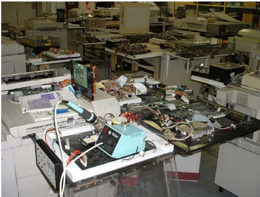
Figure 10: Testing rig for photocopiers (Courtesy: Calyx)
