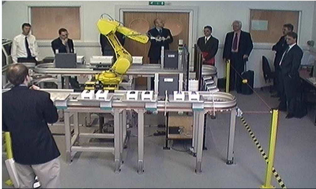
Figure 3. A demonstration to business people of how the holonic cell packs Gillette items into gift boxes after an order has been issued over the Internet.
